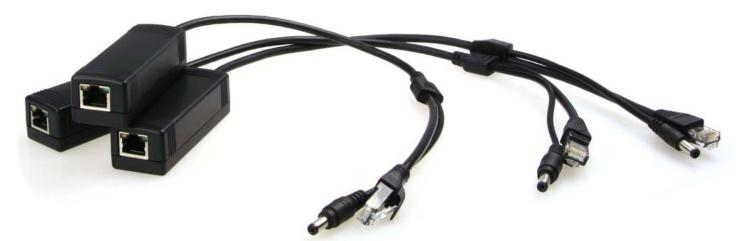
**PD41001**: 10/100M PoE Splitter/Adapter, Output DC12V, Compliant 802.3af standard, max. 15.4W, 1236 pairs
